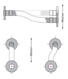
**Correct** in plane flexing Wrong out of plane flexing
