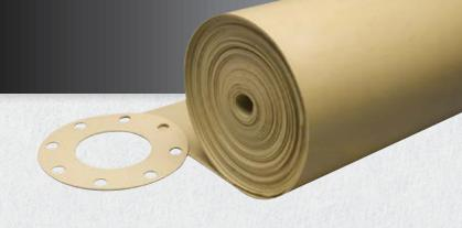
strength and is resistant to water, most salts, mild acids and other chemicals. Not suited for environments involving ozone, strong acids, animal fats, oils, greases and most hydrocarbons. Non-marking and safe to use for repeated food exposure.
